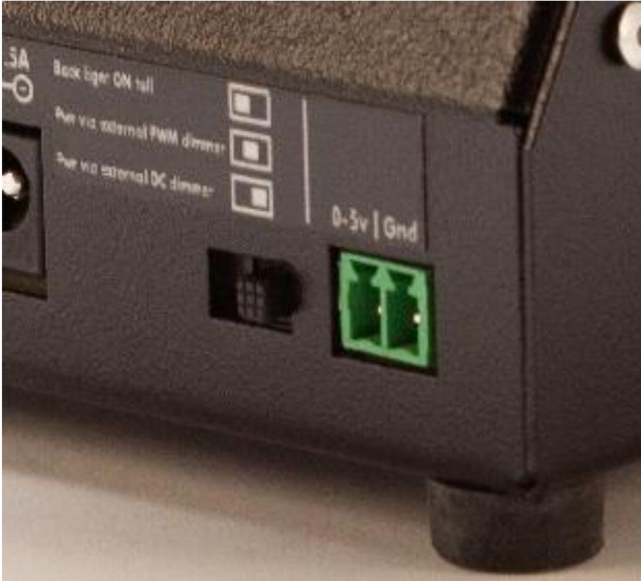
Pin1 – DC voltage from “0 to 5V” from voltage regulated dimmer **OR** “PWM” from PWM dimmer.
