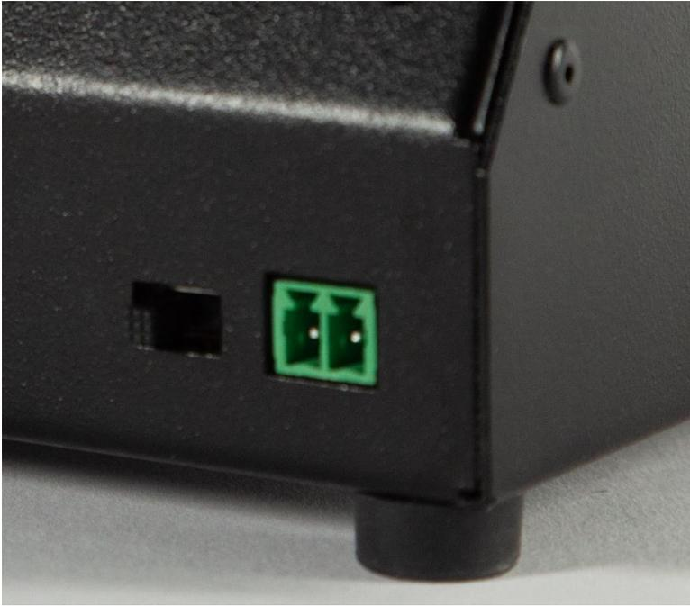
Pin1 – DC voltage from “0 to 5V” from voltage regulated dimmer **OR** “PWM” from PWM dimmer.
