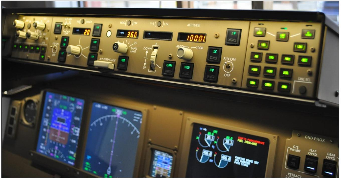
Plug the 12V power and USB into your Sim-A Avionics PC. The MCP is identified in the SYS Controller and requires no files or setup.
