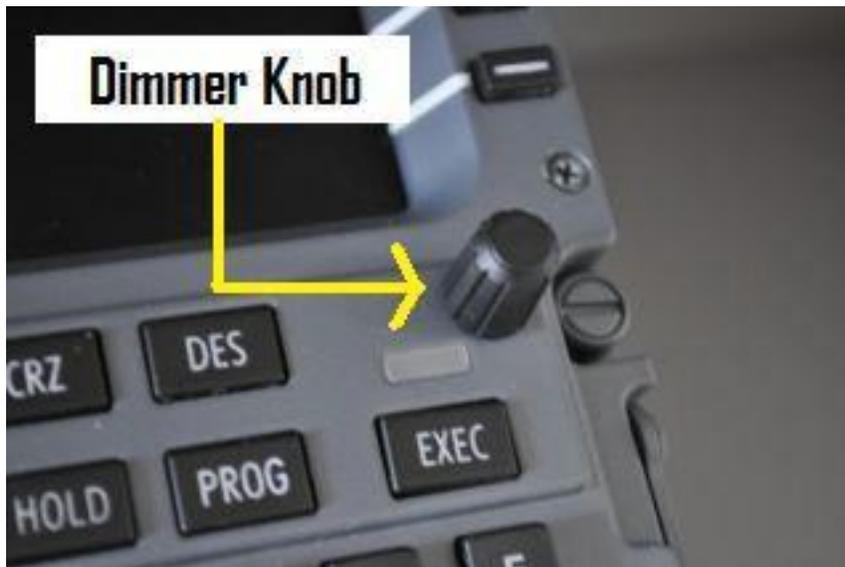
Functioning Dimmer for key backlighting and
