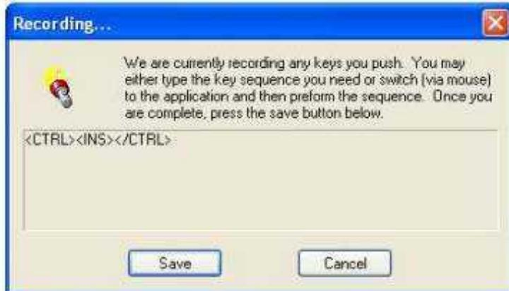
When you click on the icon to the right of the Keystroke box, the Recording screen opens. The series of keystrokes desired is entered, then the Save button is pressed. This is then named, saved in a XML-like format, and wired to a switch to control the function. That's all there is to it.
