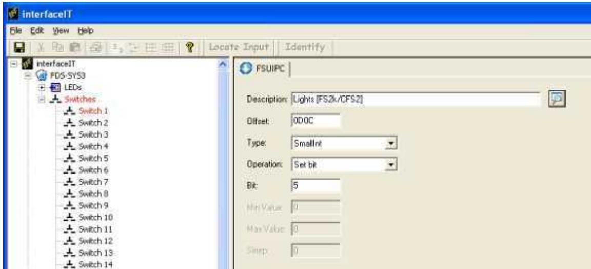
At this point we have now configured a switch to turn on the panel lights and it will be active immediately and ready for testing. If you toggle your switch (and Flight Simulator is running) you should see the panel lights go on. To configure them to be turned off, you just need to repeat the process; select the same switch, right click and add a action, “Add input action / Update FSUIPC / Off”, pick the offset, however now we want to “clear bit” for the operation and select bit 5.
